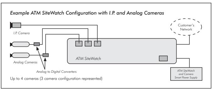
Camera connections to Smart Power Supply not shown on diagram.
